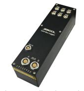
Onboard Bus Logger CANLogger-6FD, is mainly used in vehicle crash tests to collect data on the vehicle's CAN bus and provide T0 time mark. The equipment is designed according to the 6-channel standard CAN. The equipment is connected by bus. The baud rate of each channel is set before the collision. When the ARM (or SR trigger) is started, the data can be downloaded after the test.
