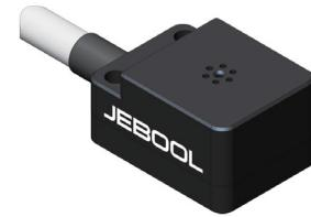
Pressure sensor DP50K, based on piezo resistance effect, zero at ambient, includes a full bridge circuit. There is resistance changed by measuring different air pressure, then the voltage signal can be converted according to the resistance difference. The reasonable MEMS process makes the sensor good linearity performance and stability. The sensor includes wear-resisting cable with default length 8m. The LEMO connector and Dallas ID are optional.
