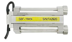
Seatbelt force sensor based on full bridge takes the principle of strain and transfers the internal tension of the belt to sensor structure. The strain structure can change resistance different, and then convert it into voltage change. The main structure of sensor is made of titanium alloy material to reduce its weight to other effects. SBF-16kN is equipped with high performance wear cable. Dallas ID and the connector depend on customers.
