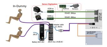
Note: DDAS is Digitization Data Acquisition System. It can record the sensor or signal data which converted by ADM modules.
