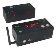
Speed Measurement Device SPS-5M, by two groups of high-speed laser sensors of front and rear installed in opposite direction, can detect the time difference of the object passing through the two sets of laser sensors. So that the speed can be calculated because the length is constant. The result can display by internal LED or external LED, and even remote PC.
