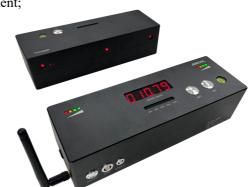
Speed Measurement Device SPS-20M, by two groups of high-speed laser sensors of front and rear installed in opposite direction, can detect the time difference of the object passing through the two sets of laser sensors. So that the speed can be calculated because the length is constant. The result can display by internal LED or external LED, and even remote PC.
