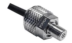
Pressure sensor AP500K, based on piezo resistance effect, zero at ambient, includes a full bridge circuit. There is resistance changed by measuring different air pressure, then the voltage signal can be converted according to the resistance difference. The reasonable MEMS process makes the sensor good linearity performance and stability. The sensor includes wear-resisting cable with default length 8m. The LEMO connector and Dallas ID are optional.
